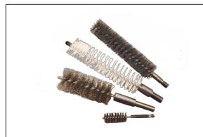
**Twisted-in-wire Brushes** are commonly referred to by our customers as twisted brushes, tube brushes, bottle brushes or pipe brushes. Twisted-in-wire brushes are made by placing filament material in between the stem wires and then twisting the stem wires tightly to secure the filament.
